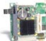
SBC1586: Headless, Low-Power PC/104 Pentium with Compact Flash, 4 COM ports, USB, and Ethernet. Boots in under 4 seconds.
