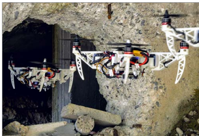
Figure 1 | Pictured are shape-shifting drones performing a gap traverse. Credit: UZH.
