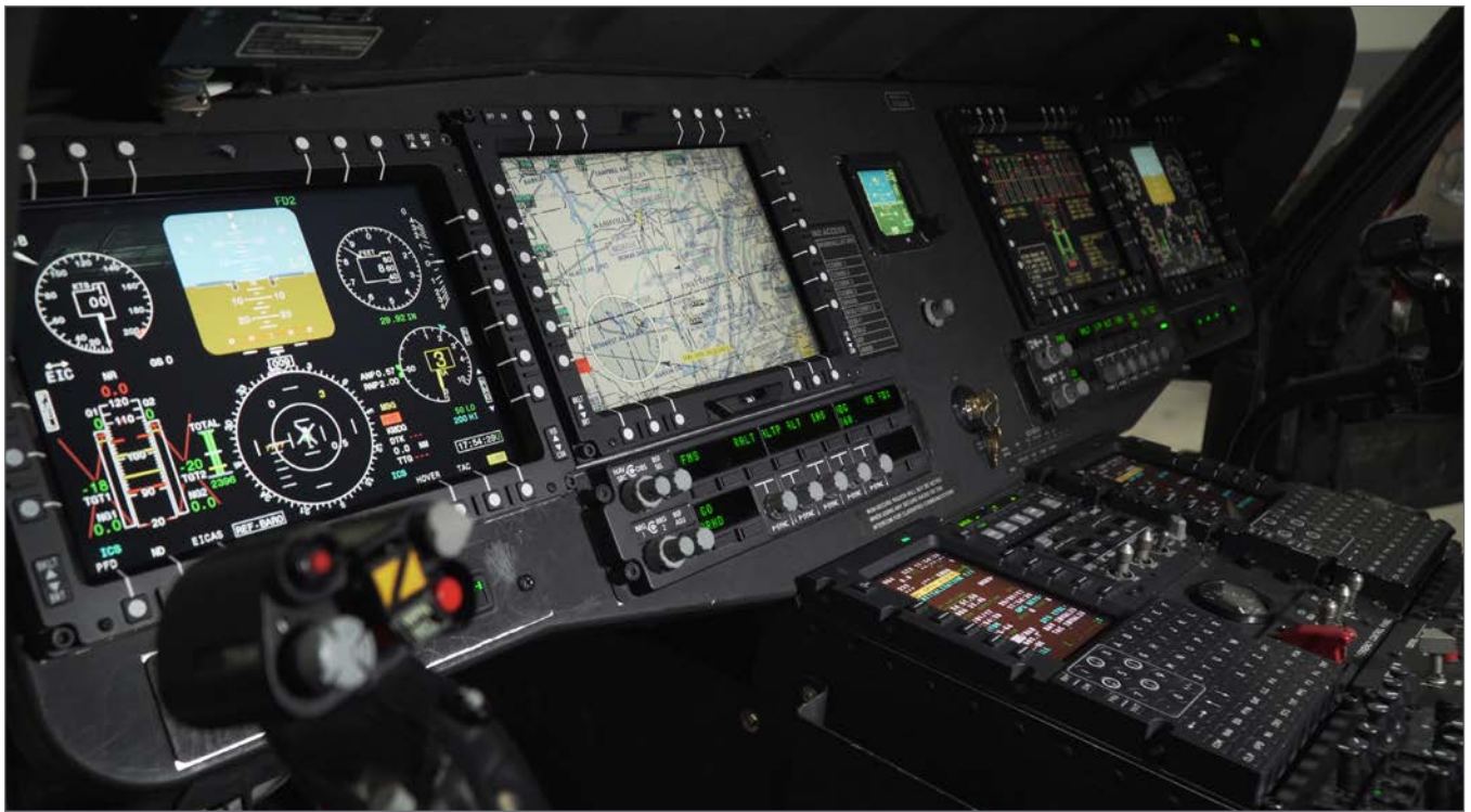
Figure 1 | Northrop Grumman's UH-60 V digital cockpit design is modernizing the Army's fleet of Black Hawk helicopters, giving pilots improved situational awareness and enhancing mission safety. Photo: Northrop Grumman.
