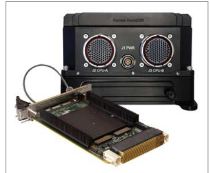
Figure 1 | The demo at the FACE TIM featured Harris's FliteScene Digital Moving Map software and Green Hills' INTEGRITY-178 tuMP real-time multicore OS running on Curtiss-Wright's Power Architecture-based VPX3-152 DO-254 safety certifiable SBC, and the Intel-based Parvus DuraCor 8042 mission computer.
