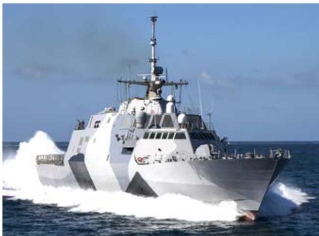
Figure 3 | The LCS's steel monohull design has 40 percent reconfigurable shipboard space. Photo courtesy of Lockheed Martin.
