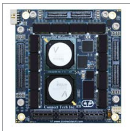
Figure 1 | The XDG024 from Connect Tech is intended to stack directly into a PCIe/104 stack for small-form-factor embedded computing applications.
