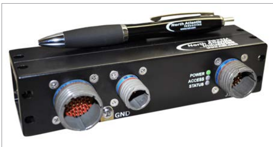
Figure 3 | Nanosized subsystem with Intelligent I/O capability connects to existing platform Ethernet networks, making data available to any system on the network.
