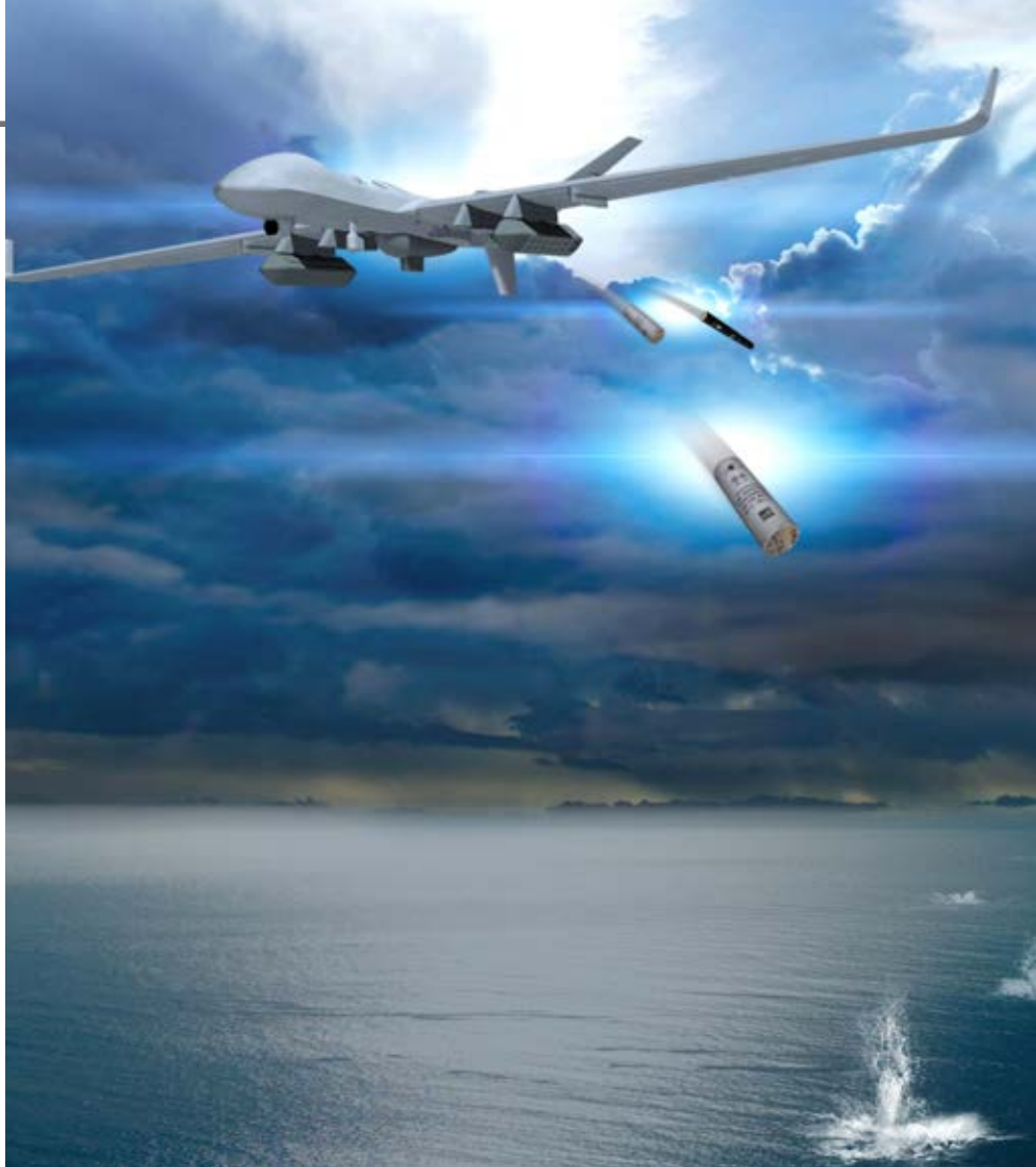
The multimission Predator B is highly modular and configured easily with a variety of payloads. Shown here, Predator B drops sonobuoys for an anti-submarine warfare mission. (Photo courtesy of General Atomics – Aeronautical Systems, Inc.)
