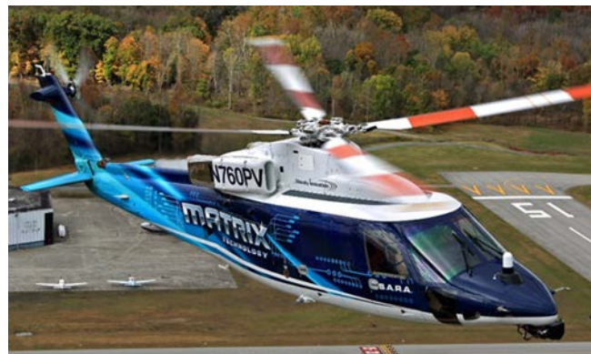
Figure 2 | DARPA's ALIAS program demonstrates its technology on a Sikorsky S-76 helicopter during Phase 2 flight tests. Photo courtesy of DARPA.
