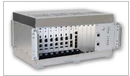
Figure 1 | Kontron's StarVX 3U blade combines dual ports of integrated 10 GbE and integrated I/Os (PCIe, USB, SATA, and other general purpose I/Os) into a single system.
