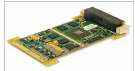
Figure 1 | The GRA113 leverages commercial NVIDIA technology on a form factor aimed at use in rugged radar and electronic warfare applications. Photo courtesy of Abaco Systems.
