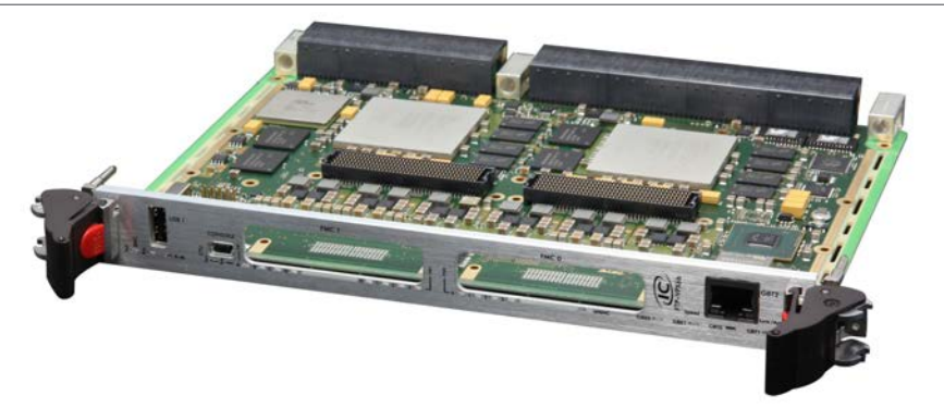
Figure 1 | IC-FEP-VPX6b featuring two Virtex-7 FPGAs.
