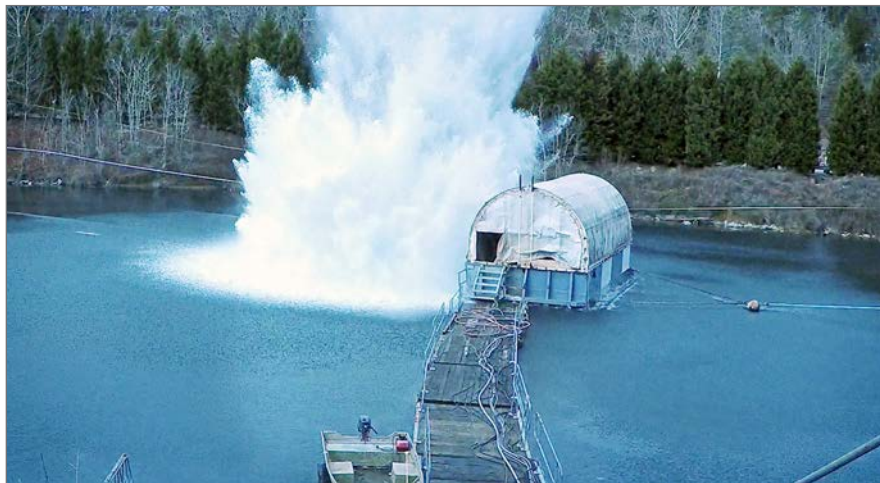
Figure 2 | Navy barge test of 4U rugged server. Effect of 60 pounds of explosives 20 feet from barge and 24 feet deep in the water. (Photo courtesy Chassis Plans.)
