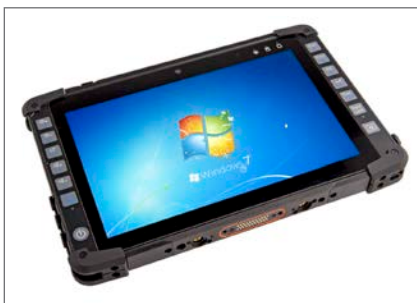
Figure 1 | The MilDef DS11 10.1-inch tablet has an IP65 rating. Photo courtesy of MilDef.
