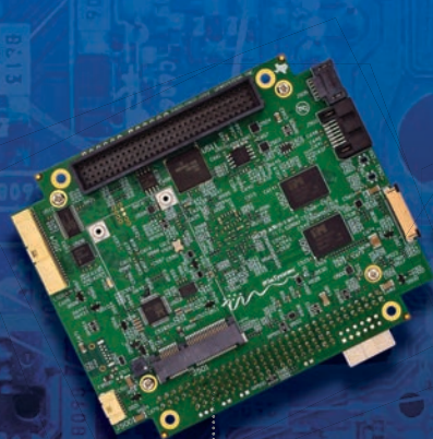
PPM-C407 Fanless E3800 PC/104 SBC Computer
