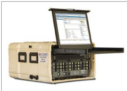
Figure 3 | Pictured is a shock-mounted 6U transit case from Chassis Plans that supports a 2U military-grade server with two multicore XEON processors, multiple PCIe expansion slots, a RAID storage unit with as much as 48 TB of disk storage, a UPS/power conditioner for assured operation in power-poor environments, and a military-grade rackmount keyboard/LCD display. (Photo courtesy Chassis Plans).
