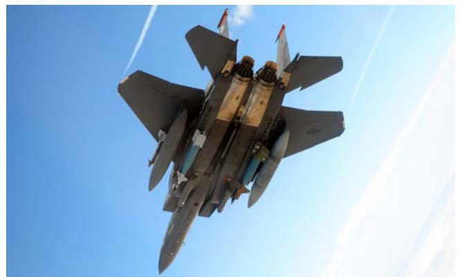
Figure 4 | An F-15E Strike Eagle flies with a Lockheed Martin Paveway II Plus GBU-12 (500-lb) LGB (left) in flight exercises. Photo courtesy of the U.S. Air Force.
