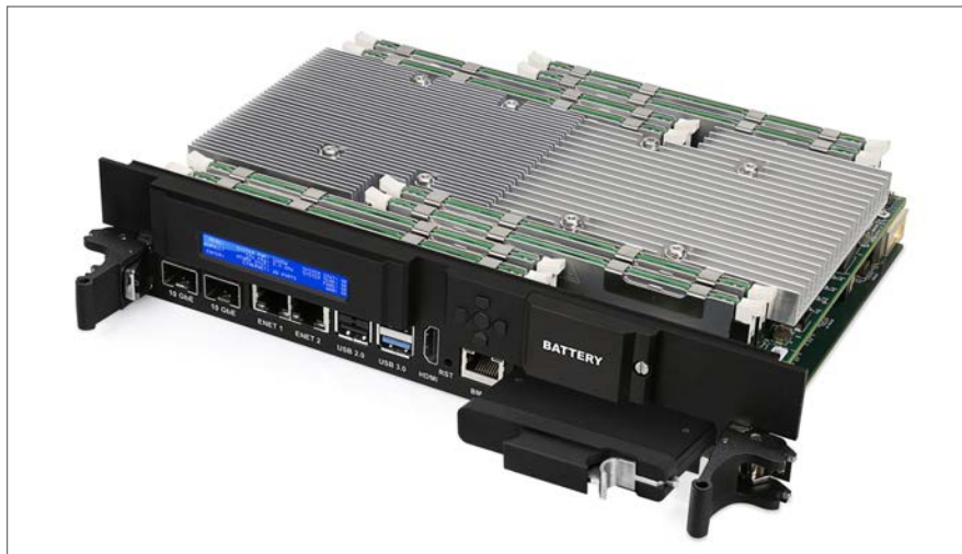
Figure 2 | Close-up of dual-processor server heat sink. This OpenVPX-based motherboard in the GMS S2U “King Cobra” server is engineered with wider fins for cooler inlet air, and narrow fins for more cooling when the air is warmer.
