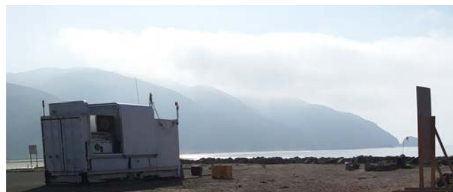
Figure 4 | IACS is a land-based survey tool that measures complex weather features and conditions that might affect laser propagation, such as optical turbulence, transmissivity, and water vapor levels. Photo courtesy of the U.S. Navy.
