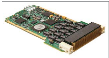
Figure 1 | Curtiss-Wright's VPX3-652 Ethernet switch is an example of an IEEE 1588-2008 PTP implementation. When configured as a transparent clock, it uses integrated timing hardware to measure and report packet transit time, enabling submicrosecond sync across the network.
