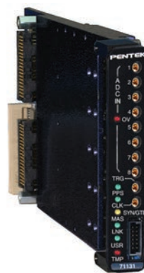
Jade Model 71131 XMC 8-channel module, also available in VPX, PCIe, cPCI and AMC with rugged options.
