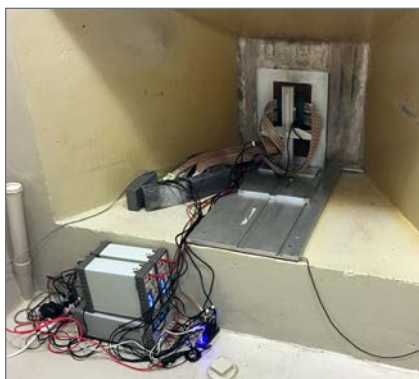
Figure 1 | TID testing in the gamma cave irradiation room at the University of Massachusetts, Lowell.
