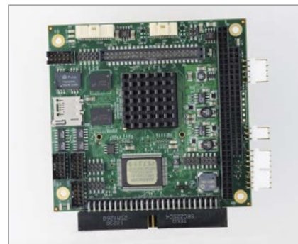
Figure 1 | WinSystems' PCM-VDX-2-512-ST is a fanless PC/104 board with the desktop-derived peripheral bus.
