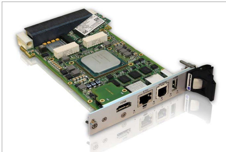
Figure 1 | The Kontron 3U VPX CPU module, based on the Intel Xeon D processor 8-core architecture, is an example of a module with the SLT3-PAY-2F2U-14.2.3 slot profile.
