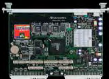
VME Bus Board Series PowerPC 750/7410 CPU Board Advme7505
