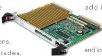
6U VMEbus SBC, MCP7447A G4 PowerPC
