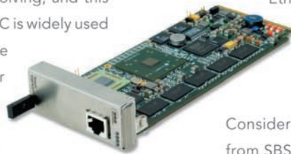
Telum TSPE01 PowerPC AdvancedMC with 1GHz G4 Processor
