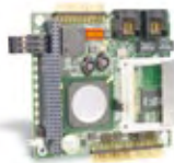
SBC1625: Low-Power ARM processor with Dual Ethernet, 4 COM ports and 24 Digital I/O on PC/104. Boots in under 14 seconds to Linux Prompt.
