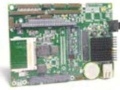
SBC4495: 486/586 EPIC CPU with GPS, Ethernet, 24 bit I/O, 14 bit A/D and D/A. Boots in under 4 seconds.
